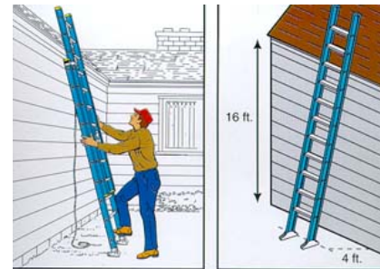
Use the 4-to-1 rule when setting up a ladder.
